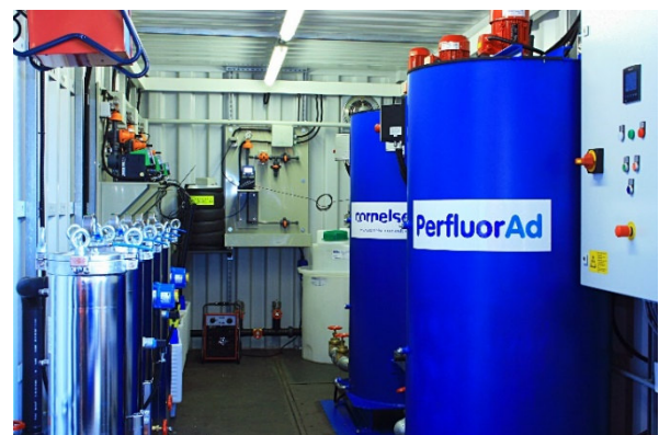
Figure 5: Mobile PerfluorAd treatment plant for the treatment of rinse water or extinguishing water
